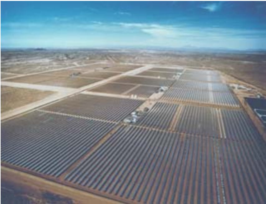
Figure 1: Aerial view of the five 30 MW e solar parabolic trough plants at Kramer Junction, California (Courtesy of KJC)
