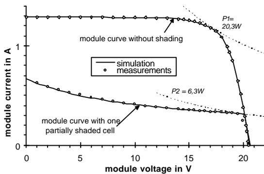
Figure 4: Comparison between measurements and simulation of the characteristic curve of a photovoltaic module with 36 cells without bypass diodes
