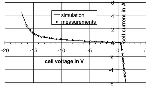
Figure 2: Comparison between measurements and simulation of the characteristic curve of an unilluminated solar cell
