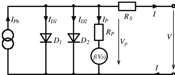
Figure 1: Equivalent circuit of the solar cell
