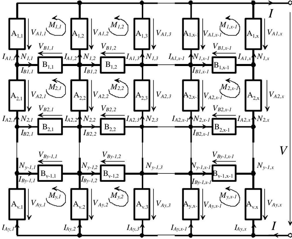
Figure 3: General model for a connection of various elements in a photovoltaic assembly
